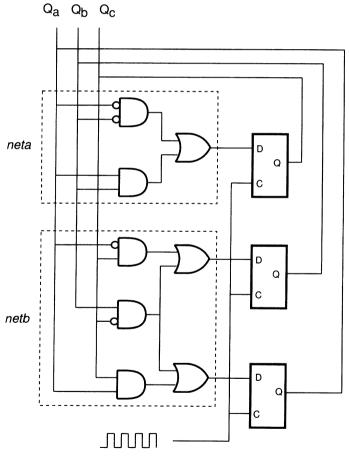
Here two combinational modules are specified as separate clauses for procedures neta and netb shown outlined in the schematic. The and and or procedures are defined in the expected way, and inv and dff are defined above. A state vector for the circuit is represented by the term
