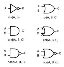
It is conventional to write inputs before outputs, so that, for example, nand(A,B,C) has inputs A and B, and output C.
