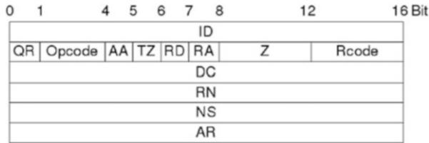
**Fig. 6.1** DNS-Header
