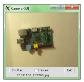
A basic camera GUI for the Raspberry Pi camera module
