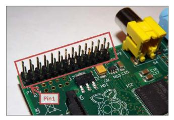
The Raspberry Pi P1 GPIO header location
