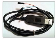
A USB to TTL serial console cable
