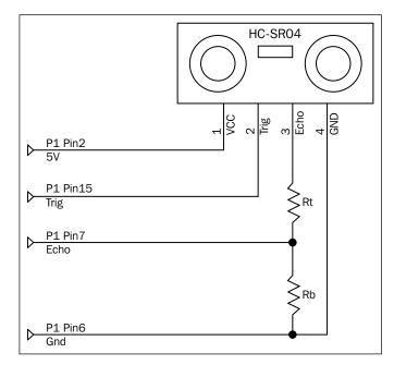
The following circuit diagram shows the connection of the sensor output:
