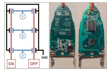
Connect the wires to ON, OFF, 1, 2, 3, and GND at suitable points on the remote's PCB (only ON, OFF, 1, and GND are connected in the image)
