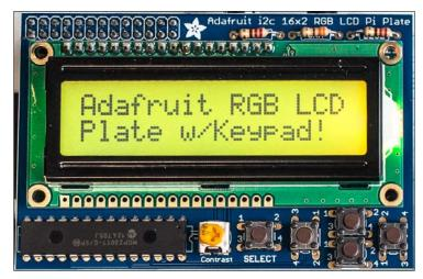
Adafruit I<sup>2</sup>C 16x2 RGB LCD Pi Plate with keypad buttons
