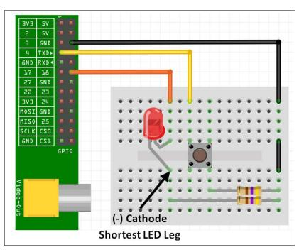
The controlled shutdown circuit layout
