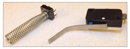
Small micro switches can be used as collision sensors
