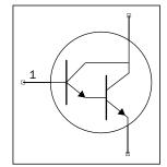
The electrical symbol for a Darlington transistor shows how two transistors are packaged together
