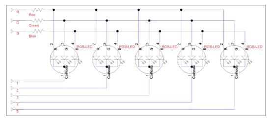
Circuit diagram for the RGB LED module
