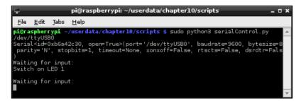
The text "Switch on LED 1" has been sent via a USB to RS232 cable from a connected computer
