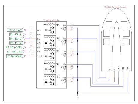
Wire the relay control pins to the Raspberry Pi GPIO and connect the socket remote control to each relay output as follows:
