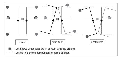
The steps to turn the Pi-Bug robot to the right are shown in the following diagram:
