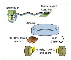
The separate parts of the Rover-Pi robot
