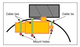
Securely fix the motors to the chassis
