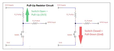
A pull-up resistor circuit
