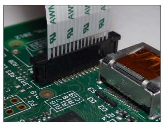
The ribbon connector for the camera module is located next to the HDMI socket
