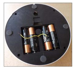
4x AA batteries provide a power source to drive the wheels
