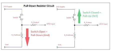
A pull-down resistor circuit
