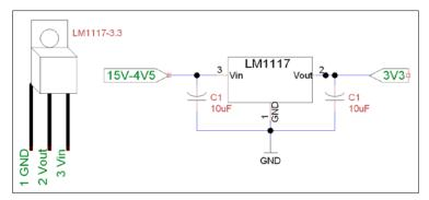
The LM1117 linear voltage regulator circuit
