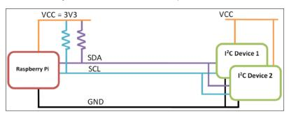
The Raspberry Pi I<sup>2</sup>C pins include pull-up resistors on SDA and SCL
