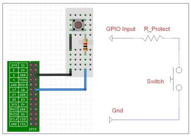
The button (and 1K ohm resistor) should be connected between pins 12 and 6 (GND)
