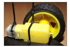
We use cable ties to secure the motors and wheels to the chassis
