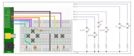
GPIO keypad circuit layout
