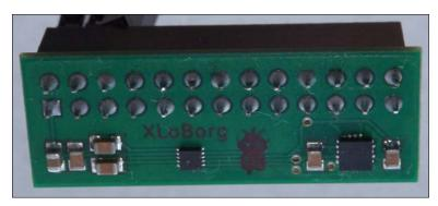
The PiBorg XLoBorg module contains a 3-axis magnetometer and accelerometer
