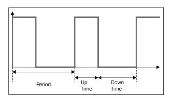
The angle of the servo is controlled by the duration of the Up Time of the PWM signal
