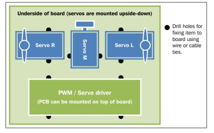
The following diagram shows the components on the Pi-Bug robot:
