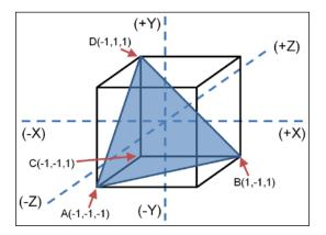
The tetrahedron placed within the X, Y, and Z axes
