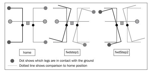
The Pi-Bug robot moving forward
