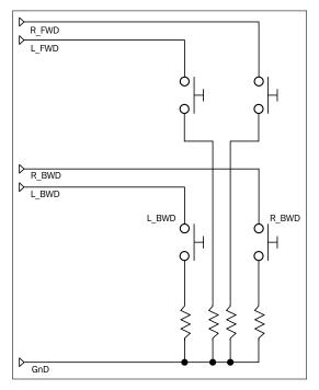
The switches should include current limiting resistors (1K ohm is ideal)
