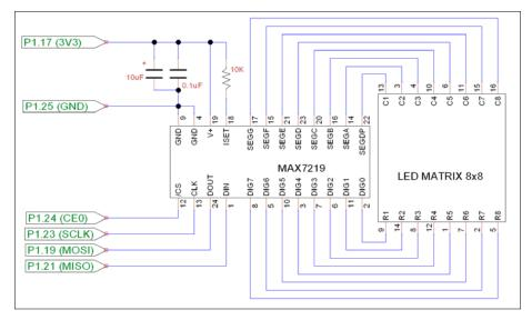
We use an 8 x 8 module connected to the MAX7219 chip as follows:
