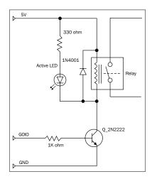
The transistor and relay circuit used to drive external circuits
