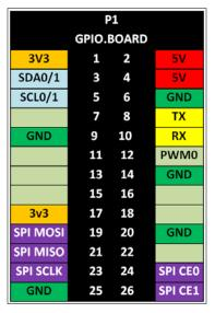
Raspberry Pi P1 GPIO header pins (pin functions)
