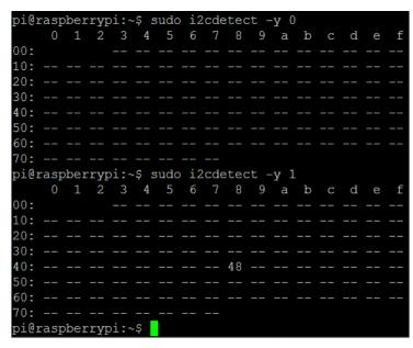
The PCF8591 address (48) is displayed here on bus 1 (on a revision 2 board)
