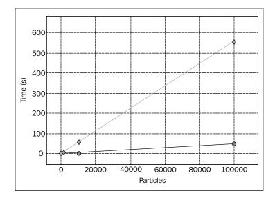
The plot shows that both implementations scale linearly with the particle size, but the runtime in the pure Python version (denoted with diamonds) grows much faster than the NumPy version (denoted with circles); at greater sizes we have a greater NumPy advantage. In general, when using NumPy you should try to pack things into large arrays and group the calculations by using the broadcasting feature.
