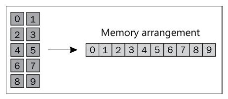
Array ordering has important consequences. When iterating a C array over the last dimension, we access contiguous memory blocks (in our example 0, 1, 2, 3 ...)while when we iterate on the first dimension, we skip a few positions (0, 2, 4, 6, 8, 1 ...). You should always try to access memory contiguously as this optimizes cache usage.
