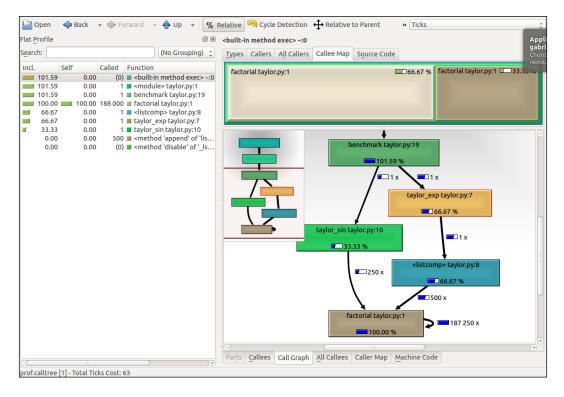
The preceding image is a screenshot of the KCachegrind user interface. On the left we have an output fairly similar to cProfile. The actual column names are slightly different: **Incl.** translates to cProfile module's cumtime; **Self** translates to tottime. The values are given in percentages by clicking on the **Relative** button on the menu bar. By clicking on the column headers you can sort by the corresponding property.
