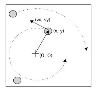
The basic feature of a circular motion is that the particles always move perpendicularly to the direction connecting the particle and the center, as shown in the preceding image. To move the particle we simply change the position by taking a series of very small steps in the direction of motion, as shown in the following figure:
