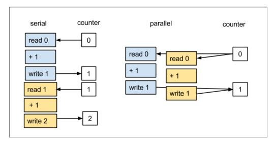
To solve this problem, we need to synchronize the access to this variable so that only one process at a time can access, increment, and write the value on the shared variable. This feature is provided by the multiprocessing.Lock class. A lock can be acquired and released through the acquire and release methods, or by using the lock as a context manager. When a process acquires a lock, other processes are prevented to acquire it until the lock is released.
