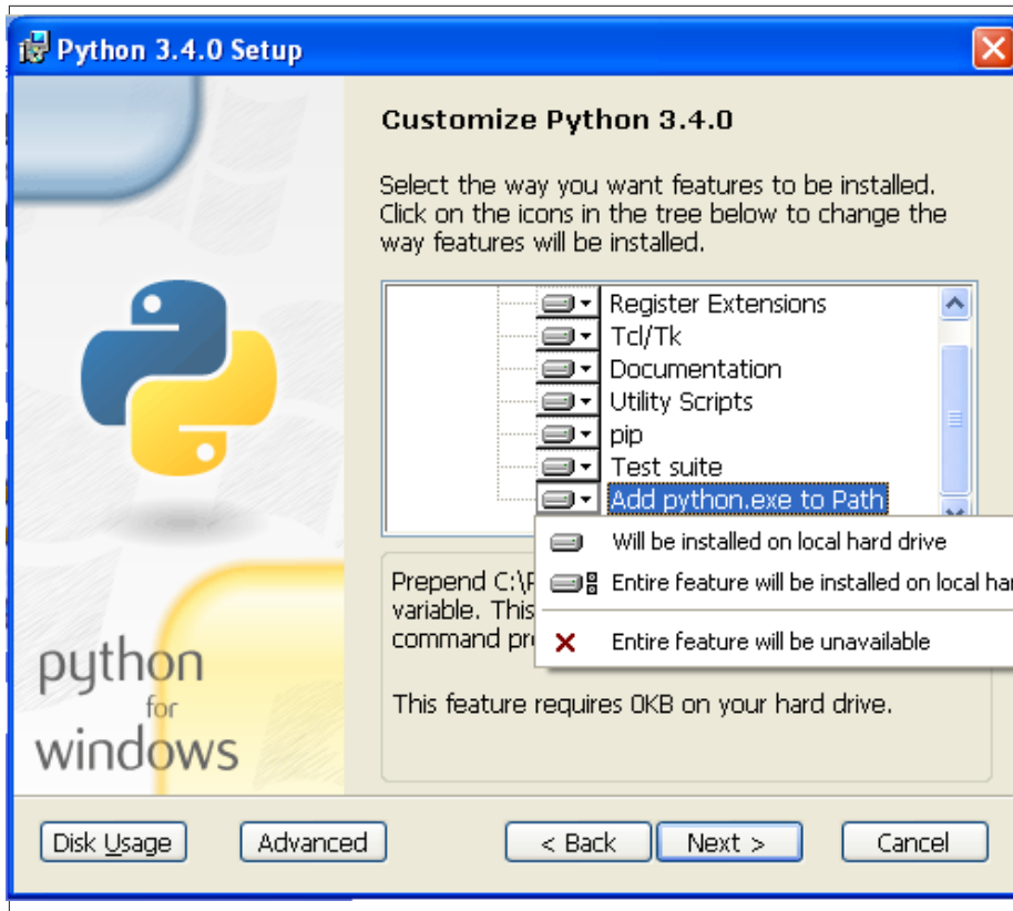
Figure **LABEL TBD**-1. Add python to the system path from the installer
