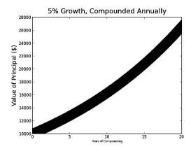
It is also possible to change the default values, which are known as "rc settings." (The name "rc" is derived from the .rc file extension used for runtime configuration files in Unix.) These values are stored in a dictionary-like variable that can be accessed via the name pylab.rcParams. So, for example, you can set the default line width to 6 points<sup>61</sup> by executing the code pylab.rcParams['lines.linewidth'] = 6.
