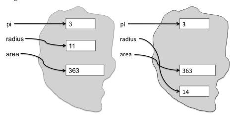
Figure 2.2 Binding of variables to objects
