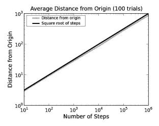
Does this plot provide any information about the expected final location of a drunk? It does tell us that on average the drunk will be somewhere on a circle with its center at the origin and with a radius equal to the expected distance from the origin. However, it tells us very little about where we might actually find the drunk at the end of any particular walk. We return to this topic later in this chapter.
