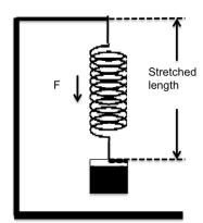
We start with a spring with no weight on it, and measure the distance to the bottom of the spring from the top of the stand. We then hang a known mass on the spring, wait for it to stop moving, and again measure the distance from the bottom of the spring to the top of the stand. The difference between the two distances then becomes the value of *x* in Hooke's law.
