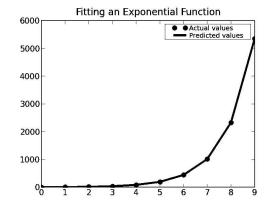
This method of using polyfit to find a model for data works when the relationship can be described by an equation of the form  $y = base^{ax+b}$ . If used on data that cannot be described this way, it will yield erroneous results. To see this, let's try replacing the body of the function f by,
