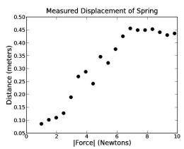
When plotData('springData.txt') is run, it produces the plot on the left.
