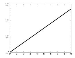
model for an exponentially distributed set of data points, as illustrated by the code in Figure 15.8. We use polyfit to find a curve that fits the x values and log of the y values. Notice that we use yet another Python standard library module, math, which supplies a log function.
