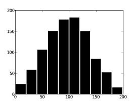
ten bins, on the left. PyLab has automatically chosen the width of each bin. Looking at the code, we know that the smallest number in vals will be 1 and the largest number 200. Therefore, the possible values on the x-axis range from 1 to 200. Each bin represents an equal fraction of the values on the x-axis, so the first bin will contain the elements 1-20, the next bin the elements 21-40, etc. Since the mean values chosen for num1 and num2 will be in the
