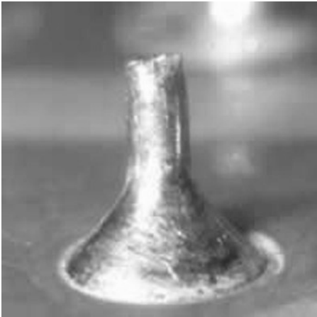
Figure 4-18. A good solder joint
